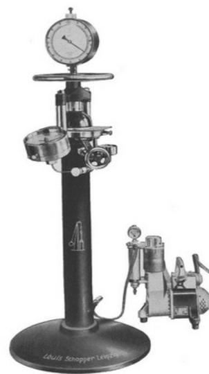
Figure 3: Schopper-Dalén Tester with air compressor [BurKor1944].
