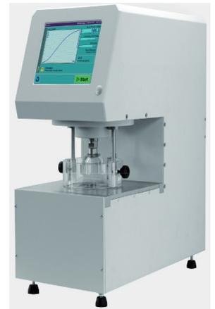
Figure 7: Modern Mullen tester with graphical display and statistical evaluation [Fra2018].
