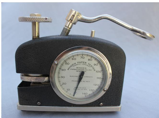
Figure 5: Paper tester (serial number 9214) from the 1940s, at that time already called Minden Paper Tester.
