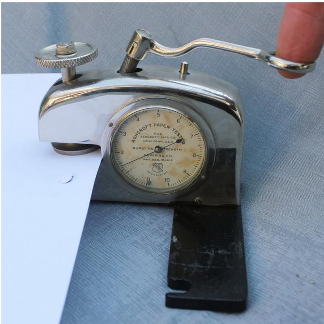
Figure 6: Tester (serial number 4164) with unlocked foot. The 80g printer paper bursts at just under 1.4 kg / cm<sup>2</sup>.
