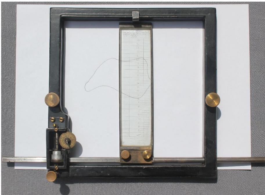
Figure 12: Mönkemöller's Glass Planimeter (Source: Collection Zerfowski).
