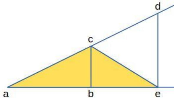
Figure 7: Proportional triangles and calculation of area of the orange triangle
