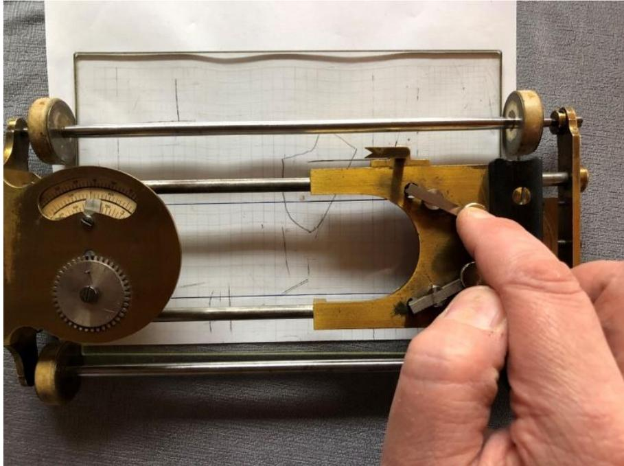
Figure 17: Operating the Köhler planimeter (Source: Collection Zerfowski)
