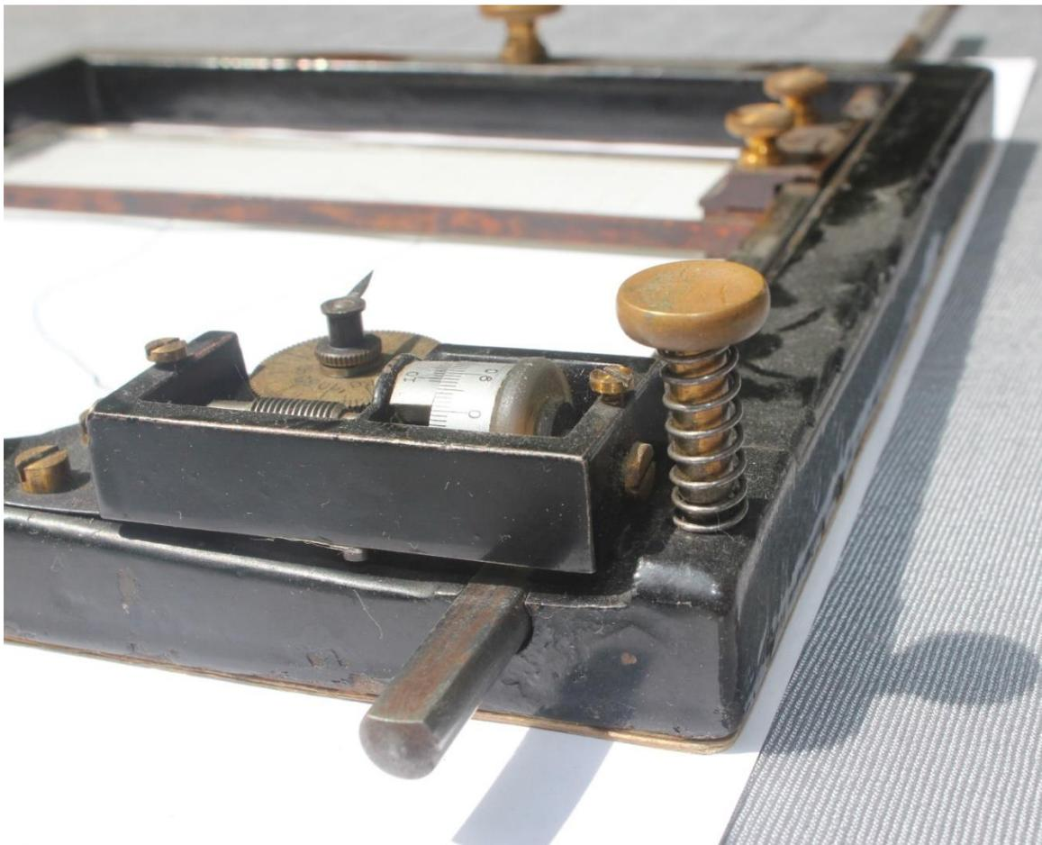
*Figure13: Mönkemöller's measuring wheel: Pressing the knob puts the wheel down on the movable metal bar (Source: Collection Zerfowski).*
