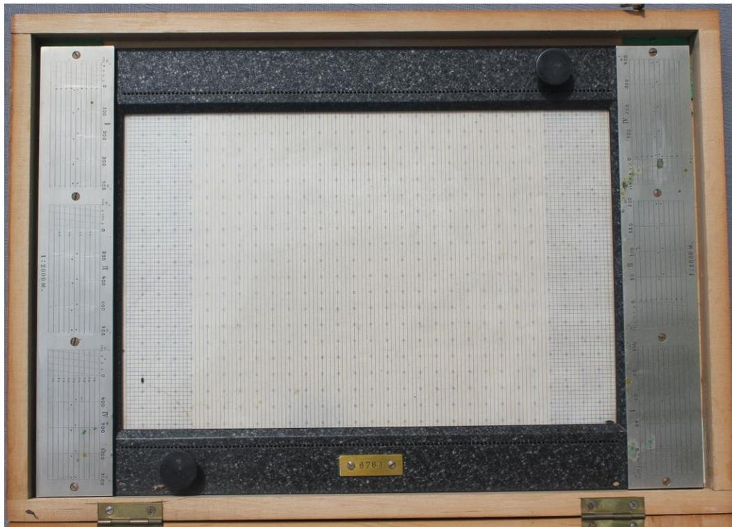
Figure 5: Harp planimeter possibly by Neuhöfer & Son, Wien. The original threads (horizontal line of thread holes are visible on the top and bottom) had been exchanged by a transparent plastic foil (Source: Collection Zerfowski).
