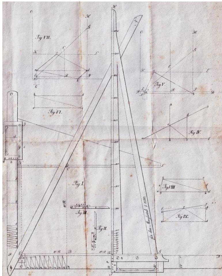
Figure 8: Drawing of Wagner's Planimeter (Source: [Wag1821], scan provided by Andries de Man)
