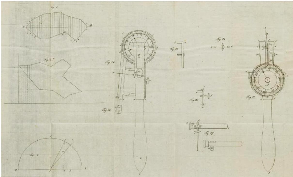
Figure 21: Oldenburg's planimeter: Measuring device, front view on the right, back view in the centre (Source: Pie1825).
