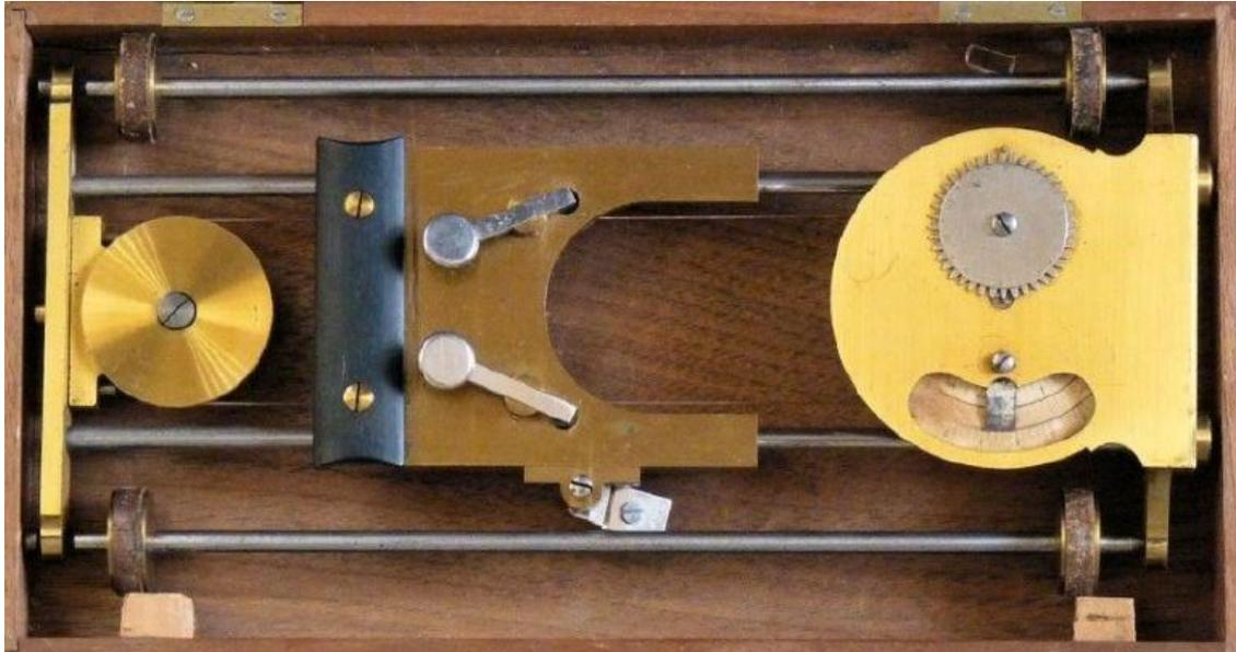
Figure 15: Köhler planimeter top view (Source: Collection Zerfowski).
