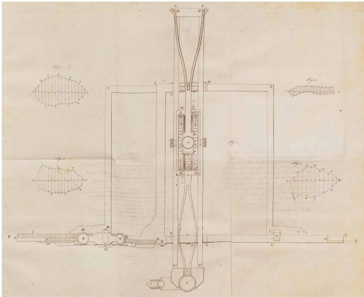
Figure 18: Zobel-Müller Planimeter, view from top (Source: [MulZob1815]).
