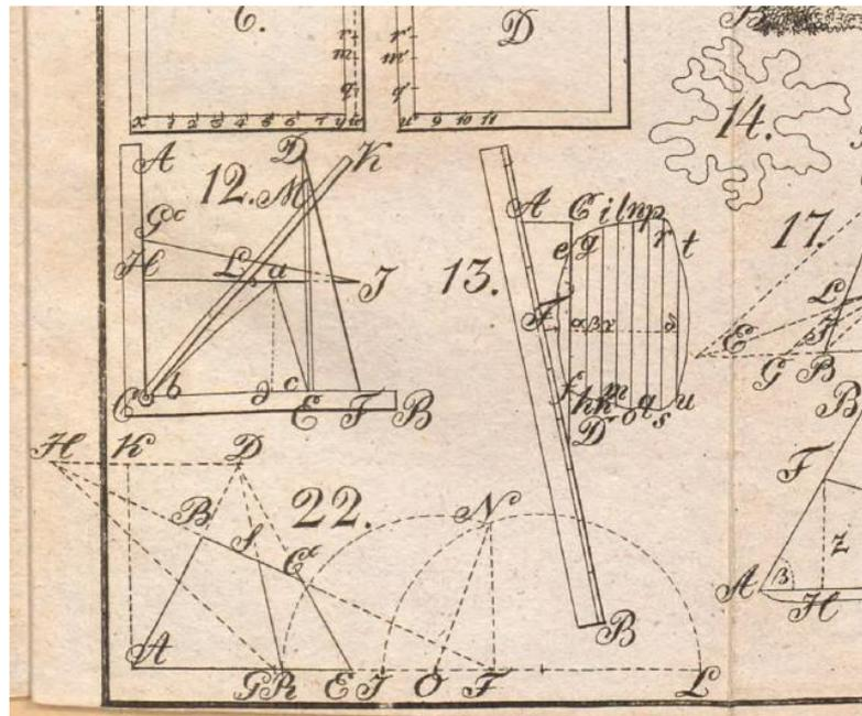
Figure 9: Netto's planimeter approach (figure no. 13) and a complex area (figure no 14). Figure no. 12 shows Wagner's planimeter. (Source: [Net1825]).
