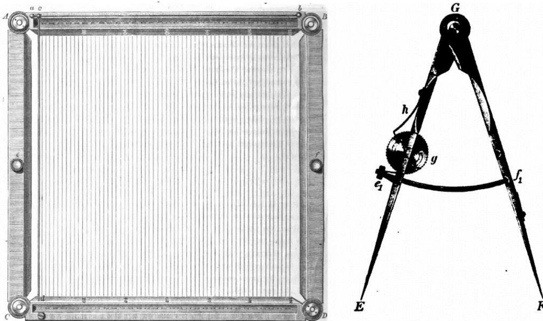
Figure 3: Oldendorp’s Harp Planimeter (Source: [Hun1862]). Figure 4: Oldendorp’s Planimeter Compass (Source: [Hun1862]).
