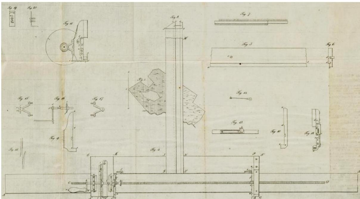
Figure 20: Oldenburg's planimeter: Stepping device for equidistant strip measurements (Source: Pie1825).
